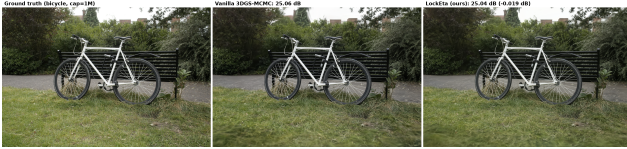
Figure 4. Iso-cap qualitative comparison on BICYCLE test view 0 at cap_max=1M . The largest perceptual gain in our table; LPIPS drops from 0.2938 to 0.2399, with the difference concentrated on the spokes, the chain, and the background fence.
